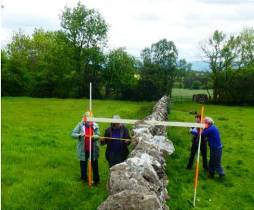
Figure 3 Volunteers using a specially-designed frame used to measure the wall profile. Photo © David Johnson
